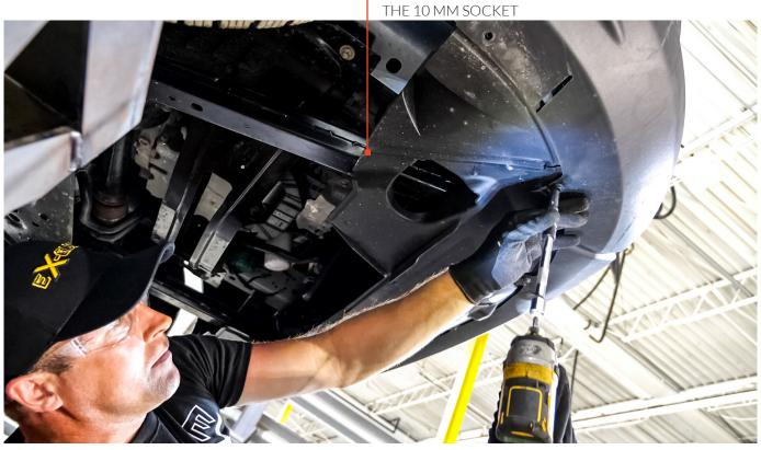
**STEP 3:**USING A 13 MM SOCKET, REMOVE THE 4 BOLTS FROM THE FRAME
