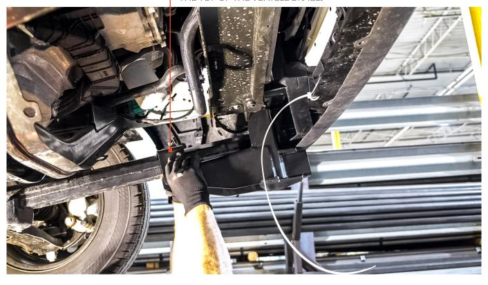
STEP 9: DRILL A 3/8" HOLE THROUGH THE TOP SIDE OF THE VEHICLE BRACE AS SHOWN
