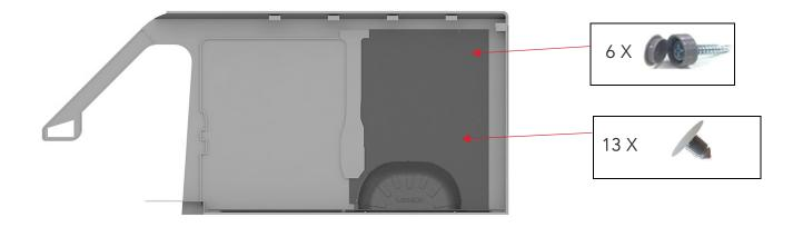
$\label{eq:Figure 9} \emph{Figure 9} \\ \emph{"Passenger Side Rear Wall Liner Installed"} \textit{This is view from Inside of the Van-Viewing from Driver Side} \\$
