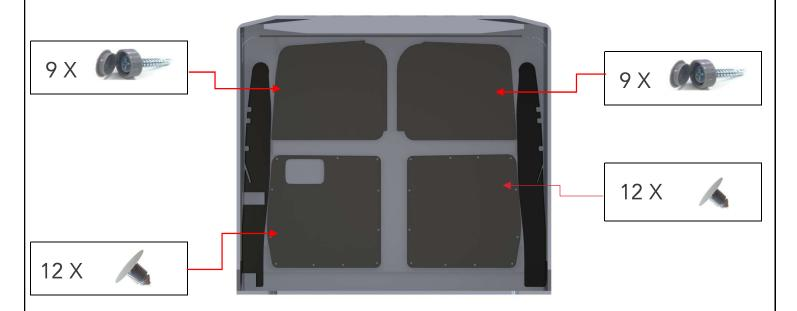
Figure 12 "Rear Door Liners Installed"
