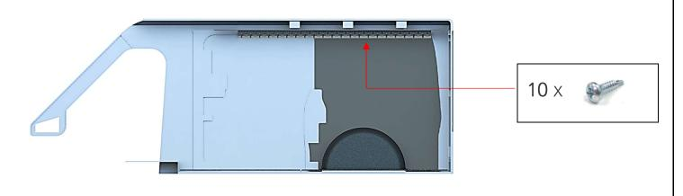
Figure 11 "Passenger side Top Sills installed"
