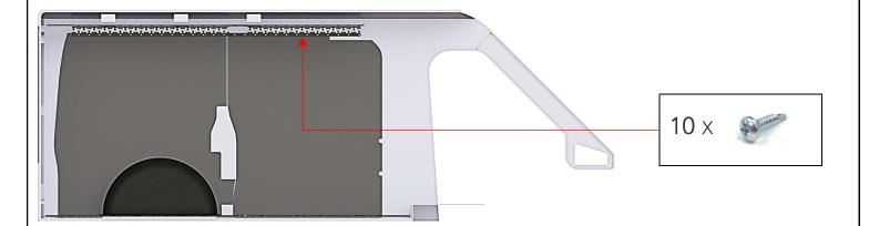
Figure 10 "Driver side Top Sills installed"
