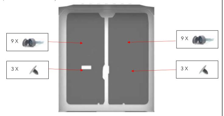
Figure 27 "Rear Door Liners Installed"
