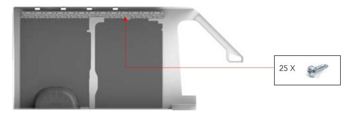
Figure 22 "Driver side Top Sills installed"
