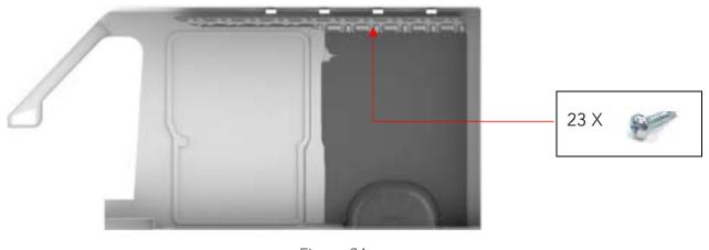
Figure 24 "Passenger side Top Sills installed"
