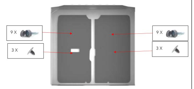
Figure 25 "Rear Door Liners Installed"
