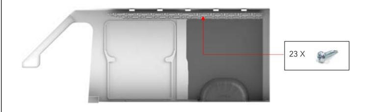
Figure 20 "Passenger side Top Sills installed"
