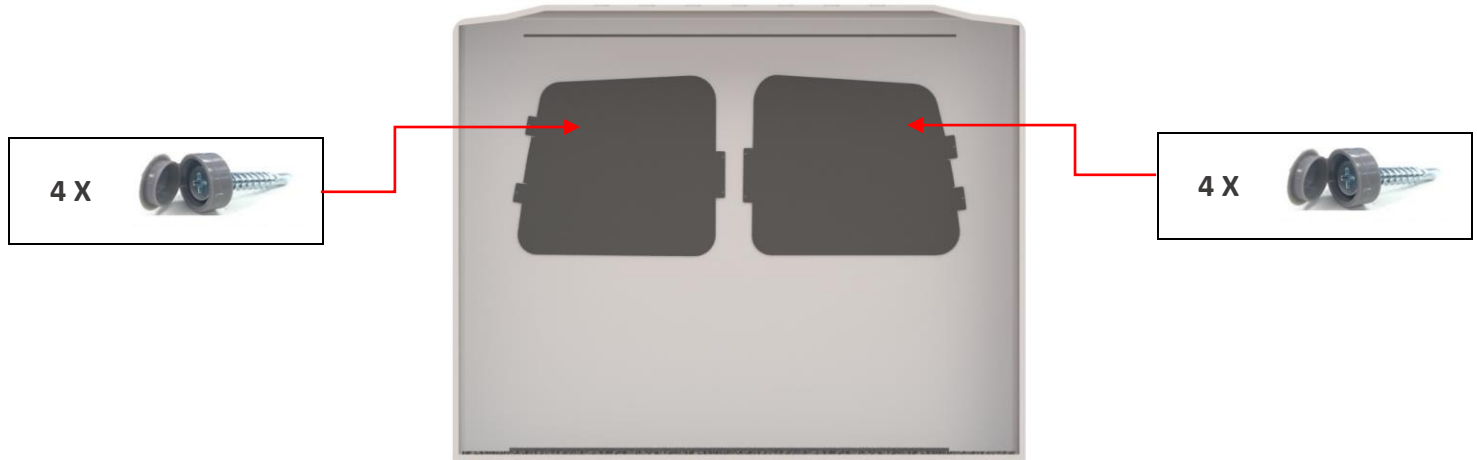
Figure 17 "Rear Door Liners Installed"
