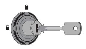
Turn key counter-clockwise 1/4 turn to unlock.
