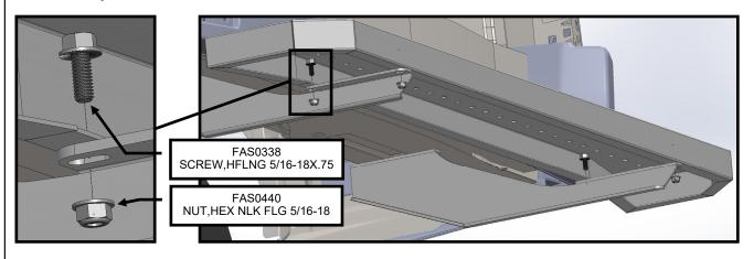
**Step 03** Adjust the step brackets to the step body is square with the vehicle. Fully tighten all fasteners.
