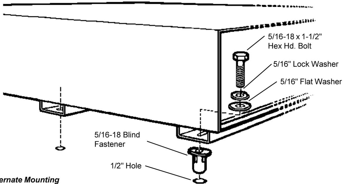
Figure 3. Alternate Mounting
