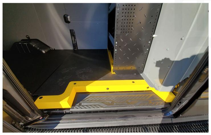
To complete the upfit, an Adrian Steel partition was added to provide driver safety, a Ranger Design shelving package to provide storage for smaller items, additional LED lighting to illuminate the cargo area of the vehicle, and 7" Luverne Grip Step running boards for safer and easy entry into the van.
