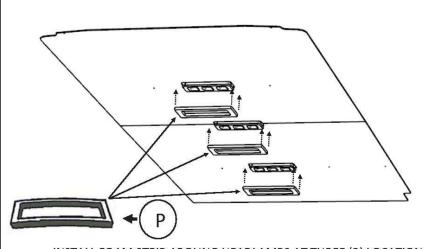
INSTALL FOAM STRIP AROUNG HEADLAMPS AT THREE (3) LOCATIONS. NOTE: DO NOT REMOVE ADHESIVE BACKING UNTIL BEZELS ARE IN PLACE
